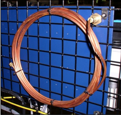
Grease Line at Pneumatic Assembly
